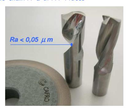
mirror flute surface left by a **SUPERFIN** wheel compared with a standard finishing Picture:
