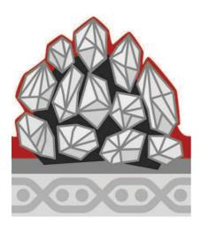
The compact grain (CG) consists of many abrasive grains and reactive filler, which are bonded to each other before adding them to the tool. During grinding, individual worn particles break out of the compact grain, exposing the underlying abrasive particles with new, sharp cutting edges. As a result, tools with compact grain do not clog even with softer or smearing materials.
