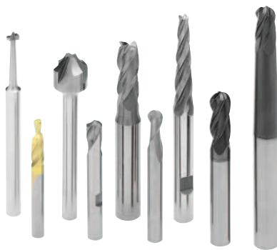
In addition to rotary burrs, we also produce tungsten carbide milling tools in special shapes and sizes for stationary applications. We supply these milling cutters with a maximum diameter of 20 mm and a maximum length of 250 mm; they differ from our extensive standard range in their shape, tool material and geometry (rake, clearance and helix angles).
