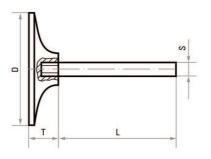
The specified maximum permissible speeds apply for a maximum overhang length  $L_{\rm 0}$  of 20 mm. The maximum permissible speed must be calculated separately for other overhang lengths.
