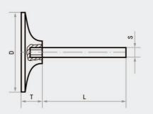
The GTH abrasive disc carriers with diameters of 18 and 30 mm have lnox hooks. Hooks with a diameter of 45 mm and greater are made of polyamide.
