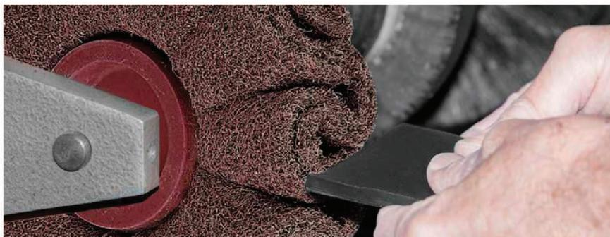
LUKAS mops of abrasive fleece are packed together on a shaft to create rolls of different widths. By adding water or low-viscosity oil, you can further boost the service life of this tool: Water produces matt surfaces on almost all metals and very matt surfaces on aluminium, while oils give a silky lustre finish.
