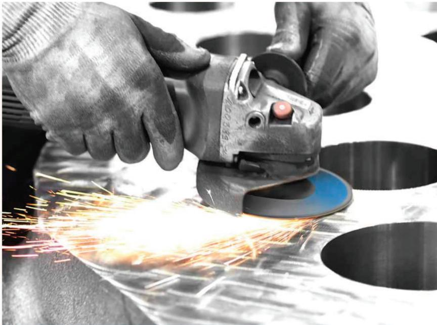
LUKAS NAWAROFLEX® lamellar flap discs have a backing plate made of renewable raw materials. Although made of paper, these special eco-friendly backing plates are nevertheless very sturdy and offer enough stability for hard grinding applications.
